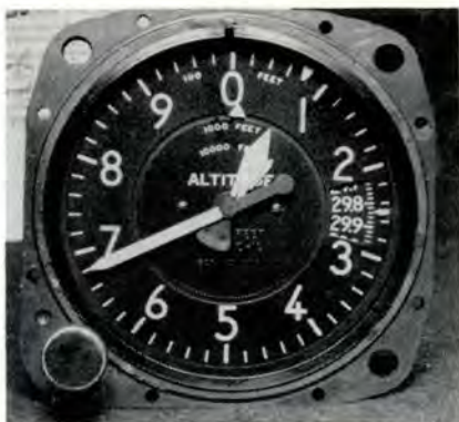
Even under ideal conditions, seven seconds are required to read the standard altimeter. During this time a jet might move 3600 feet along its flight path, and 600 feet downward.
