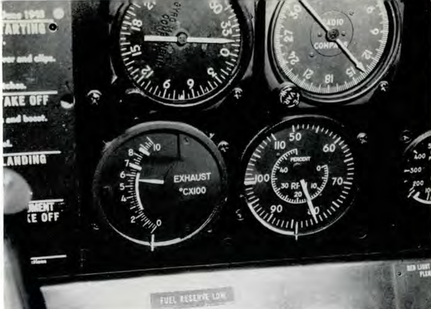
Even under ideal conditions, seven seconds are required to read the standard altimeter. During this time a jet might move 3600 feet along its flight path, and 600 feet downward.
