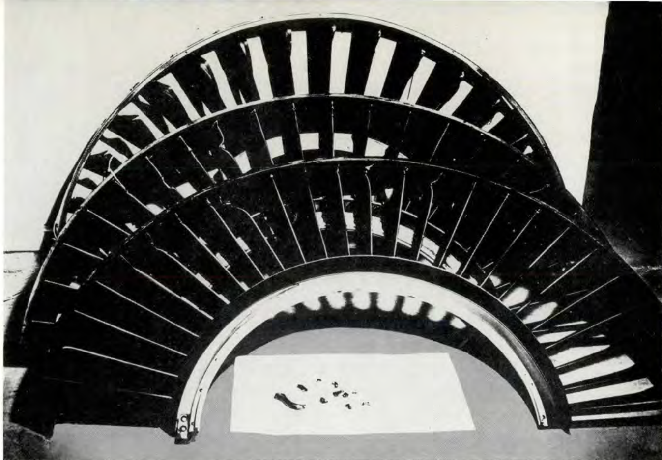
Forty per cent of all jet engines received for overhaul suffer from foreign object damage—sometimes small tools.
